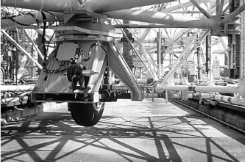
Figure 7. Test equipment for evaluation of the friction properties of concrete pavers at NASAs Aircraft Dynamics Landing Facility (ADLF) in Langley, Virginia.
