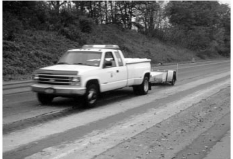
Figure 4. ASTM E 274 Test Equipment consists of a truck and trailer assembly. A tire within the trailer is towed a given speed, locked, and skidded across water dispensed on the pavement in front of it.
