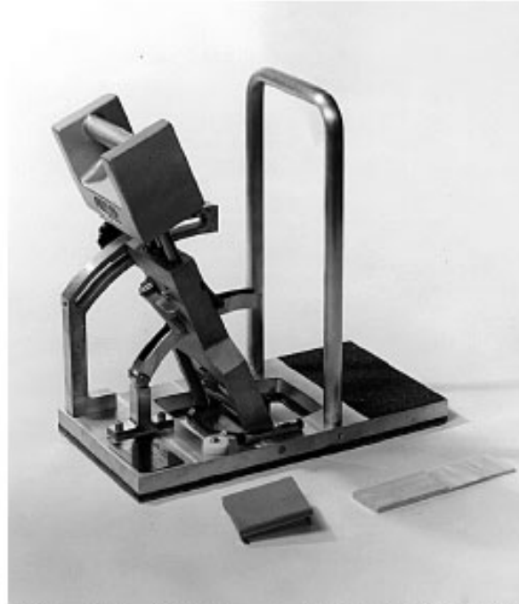
Figure 2. The NIST-Brungraber Mark II Tester for Slip Resistance
